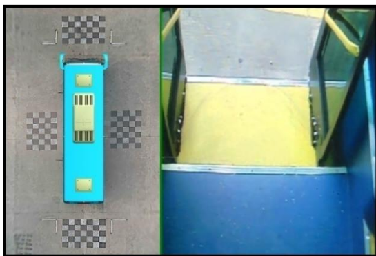
Figure 3.5 When the lower door is opened, the lower door monitoring area is displayed (5-way device version)
